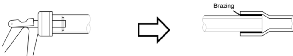
Figure 3-3.2: Expanding copper piping ends
