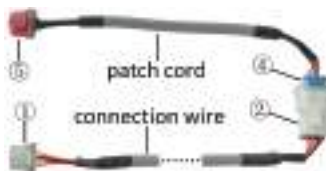
Fig. D: Schematic diagram after the connection wire and the patch cord have been connected: connect the terminal ② of connection wire and the terminal ④ of patch cord
