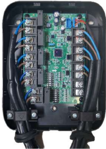
Figure 5.3 Sketch map for wire-pressing
