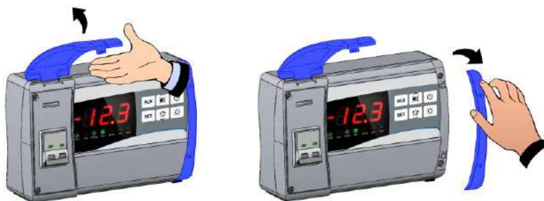
Fig. 1: Lift the transparent door that protects the differential magneto thermal circuit breaker and remove the cover for the screws on the right side.
