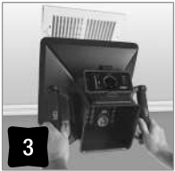
Capture airflow readings
